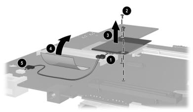
Removing the Modem Board
